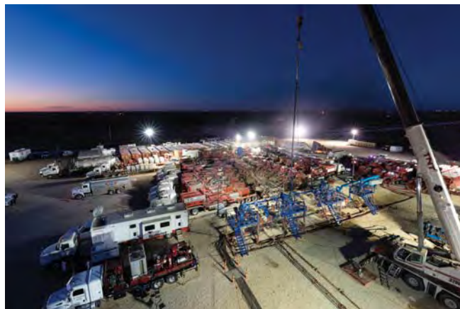
Photo: Chevron has implemented a factory development strategy in the Permian Basin, utilizing multiwell pads to drill multiple horizontal wells.
