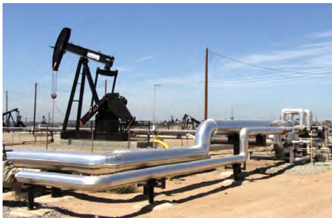
Photo: The company's industry-leading expertise in steamflood operations has resulted in more than a 60 percent crude oil recovery rate at the Kern River Field in California.
