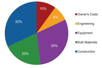
Figure 4.9: Average Cost Breakdown of Liquefaction Project by Expense Category
