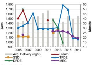
Figure 5.12: Average Delivery and Cost per Cubic Meter in Ordered Year by LNG Carrier Type, 2005–2017
